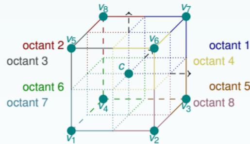
How to define advanced geometrical configurations ? with subdivision mesh gen.
